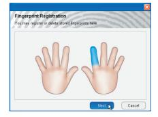
4. You will be prompted to swipe your finger across the sensor at least three times to get a good reading. Use a smooth, even movement and draw the finger or thumb back towards yourself while applying steady pressure to the sensor. Each swipe should take around a full second or more to complete. When three valid readings have been collected you will be returned to the fingerprint registration screen.
